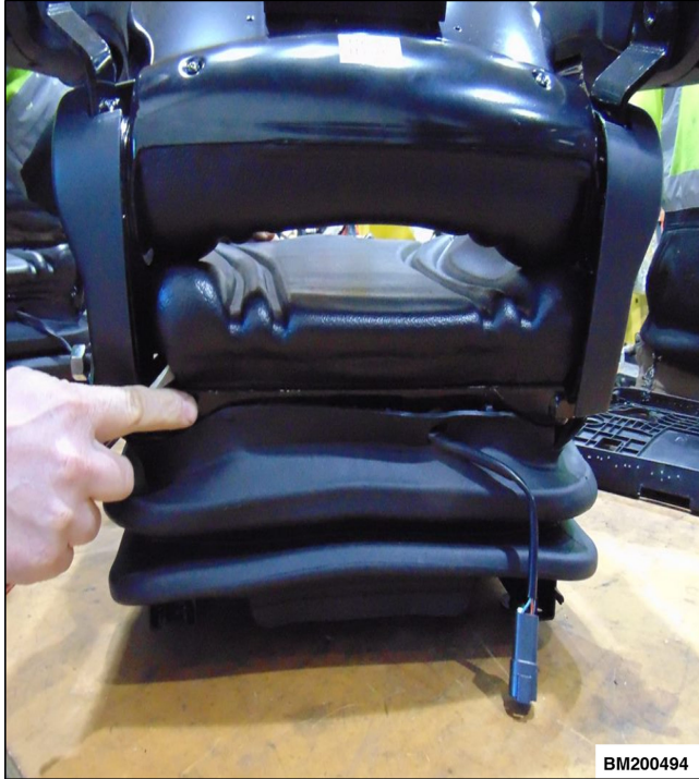
Figure 113. Pry from left side
